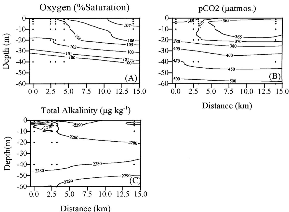
Fig. 3. Vertical sections of (A) oxygen, (B)  $p\text{CO}_2$  and (C) total alkalinity during the transect of stations across the bloom of *Emiliana huxleyi* on 30 June 1994. The symbol • indicates the sampling depths from station 27 (at left) to station 31 (at right). Positions as in Fig. 1.
